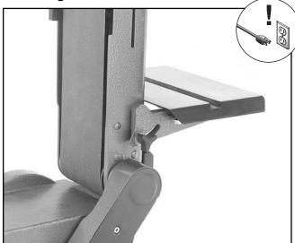
Figure 20. Installing the table for belt sanding.
